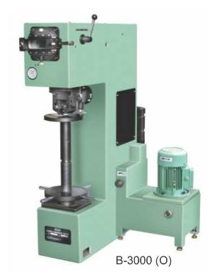
Basic machine design & operation similar to B-3000 (H). In addition 'Optical Device' with 14 x magnification provided in front of project dia of ball impression on glass screen with a micrometer measuring system with 0.01mm accuracy. The indentor swivels & projects dia of ball impression immediately after unloading operation which avoids additional time for measurement of ball impression.
